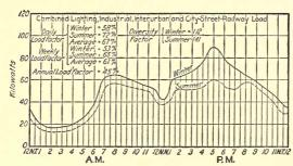
Fig. 76.—Typical 24-hour load graph for a combined lighting, industrial, interurban and city railway load.
